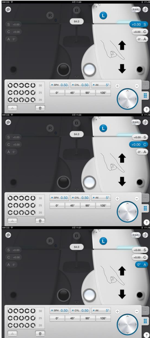
[Fig 40] Adjustment of the SPH-CYL-AXIS Value (Left)
