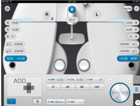
[Fig 47] Near Distance Cross Grid Test
