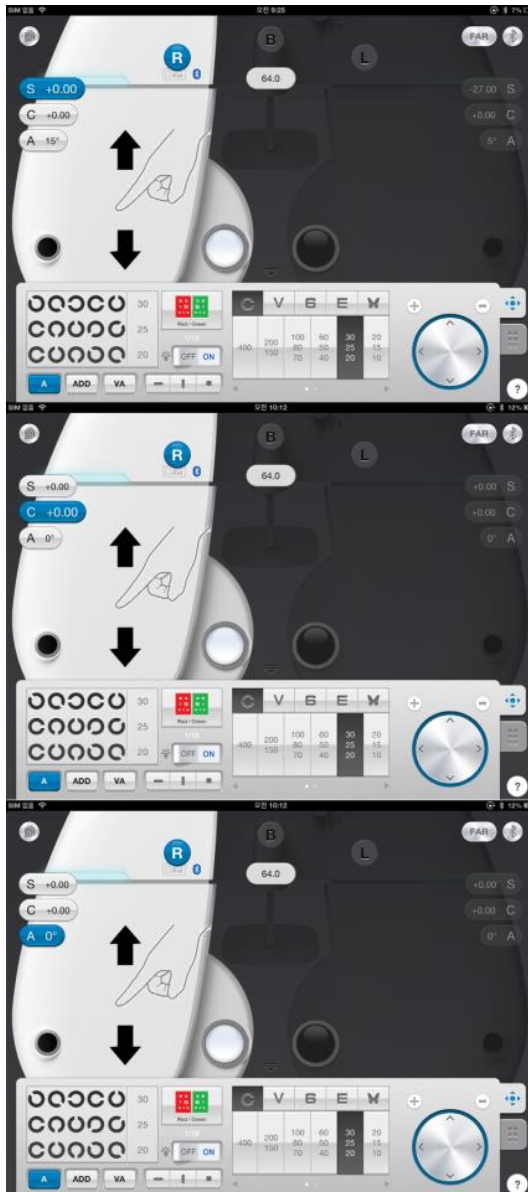
[Fig 35] Adjustment of the SPH-CYL-AXIS Value
