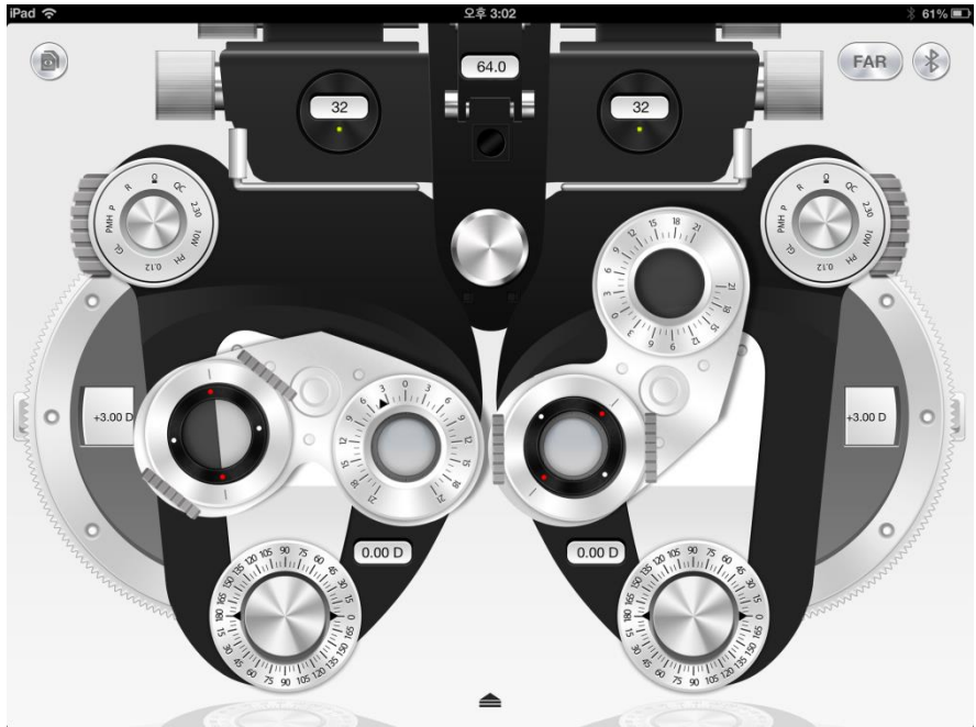
[Fig 31] Set the Risley prism (left) and the Jackson cross cylinder (Right)
