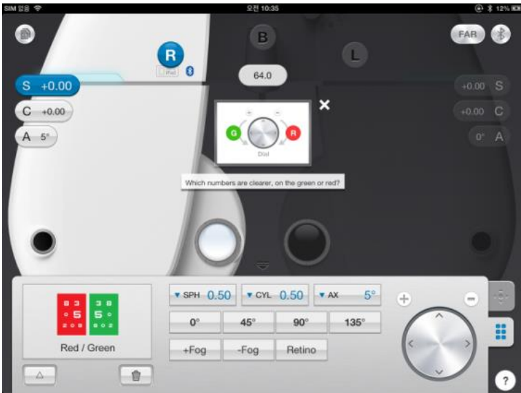
[Fig 36] Red/Green Balance Test for Monocular
