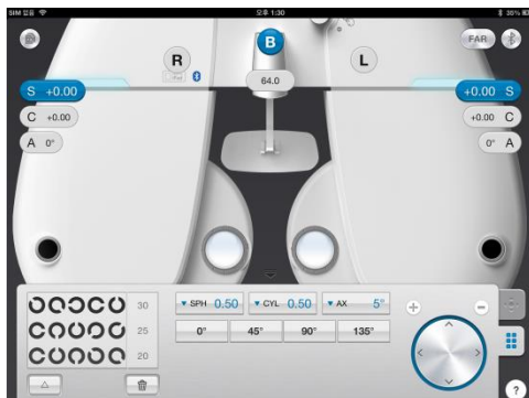
[Fig 45] Check the Power of Glasses for the Binocular
