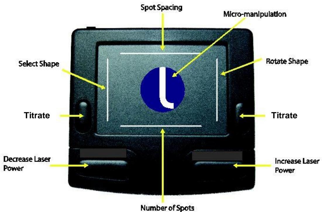
Fig. 9 The Array LaserLink Touchpad
