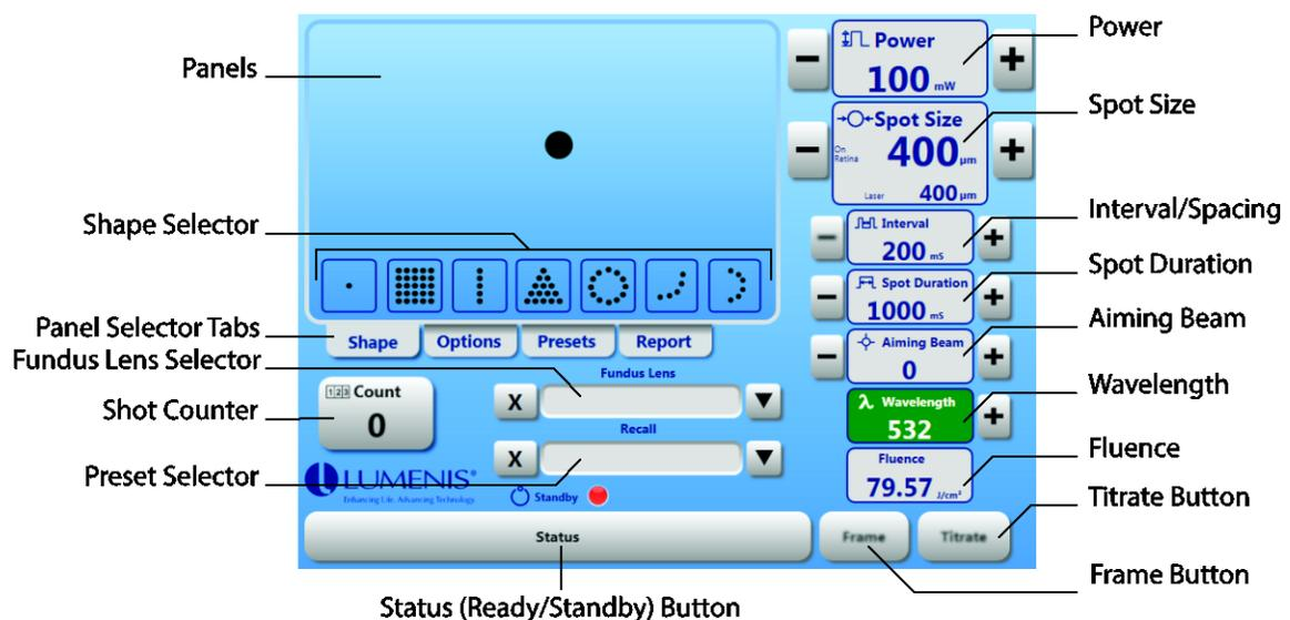
Fig. 8 The Array LaserLink Touchscreen
