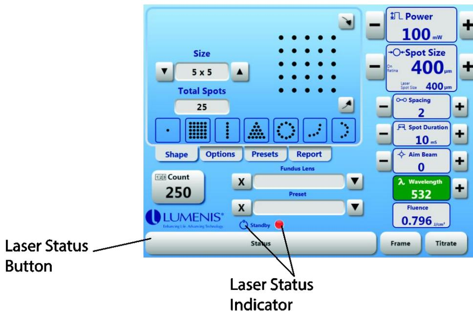
Fig. 29 Laser Status Button and Indicator
