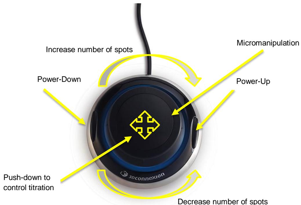
Figure 10 – The Array LaserLink 3D Mouse controls
