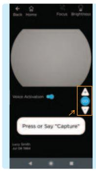
If using manual focus, use the buttons on the right-hand side of the screen to increase or decrease the focus by one diopter increments until the image is clear.
