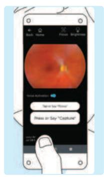
The correct working distance is reached when the entire field of view is filled with the retina without any dark spots and shadows. If you feel the need to readjust focus, tap the focus button one more time for a clear, sharp image.
