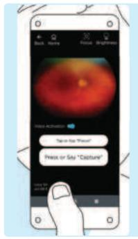
The correct imaging distance is reached when the retina completely fills the imaging window.
