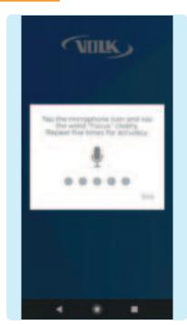
To train the device, tap the microphone icon and repeat the word "Focus" and "Capture" five times each. A confirmation screen will appear when the set up is complete.
