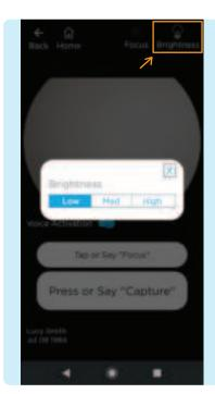
To adjust the brightness, select the \_Brightness icon. Start with the lowest brightness and increase as needed.
