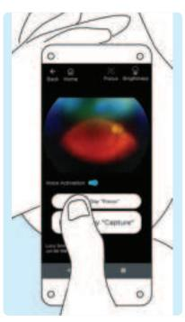
Locate the retina, which can be seen as a small reflection within the pupil. If Focus-Assist is enabled, tap the focus button when you locate the optic disc. Now that the focus is locked for this eye, you can readjust the camera position if needed.
